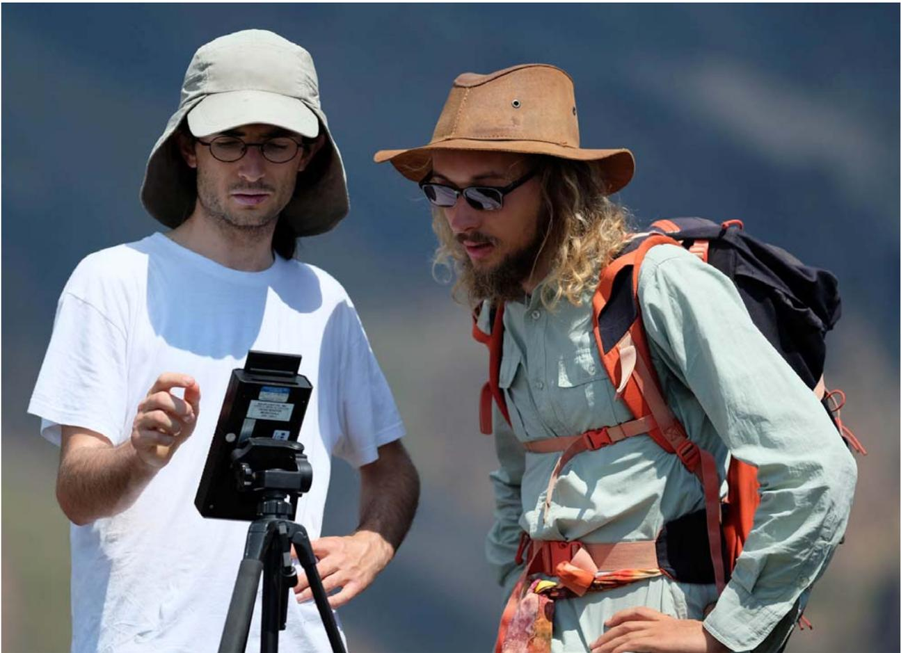
**Figure 8.** Luca Terray and Simon Bufféral performing analysis of the aerosols in the volcanic plume by using a Microtops II sun radiometer at the station Schiena del'Asino, elevation 2100 m, on July 12, 2018
